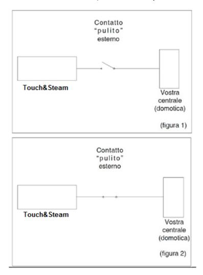
Once the remote function has been enabled, as soon as the remote external contact goes from open to closed, the Hammam will start up.
