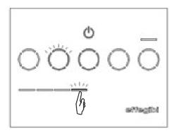
**VERY HIGH** for water harder than 30°f – De-scaling indicator after 700 hours
