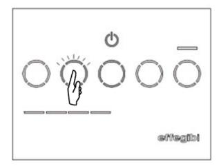
Set the desired value using function keys 1, 2, and 3
