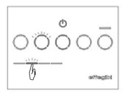
MEDIUM for water hardness between 10° and 20°f; – De-scaling indicator after 4375 hours
