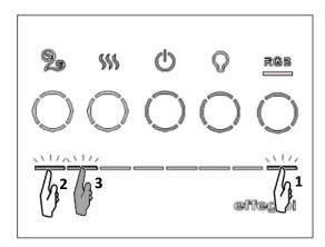
Press, in order, function key 3, function key 1 and then hold down function key 2 until the icon "O" comes on (do not hesitate between pressing the keys).
